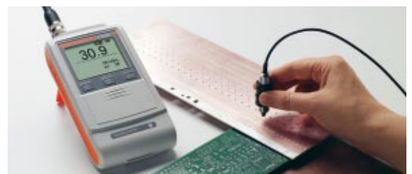
ISOSCOPE® FMP10 using the probe FTA3.3-Cu – printed circuit boards, copper boards
