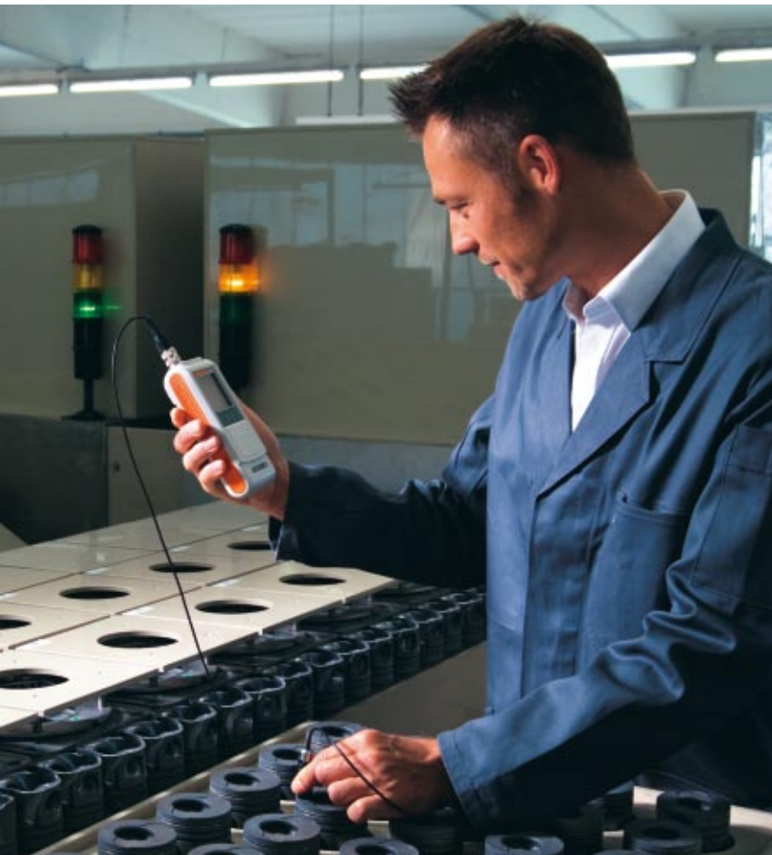
Quality monitoring on engine pistons immediately after the manufacturing process using the FTA3.3H probe
