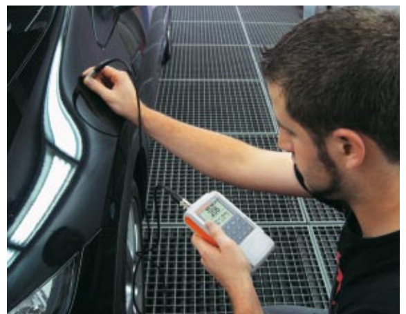
Paint coating thickness measurement using the dual probe FD10
