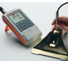
DELTASCOPE® FMP10 –zinc on iron using the probe FGAB1.3
