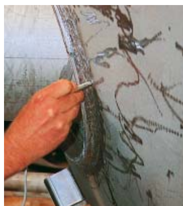
Figure 2: Measurement of the ferrite content at a weld seam
